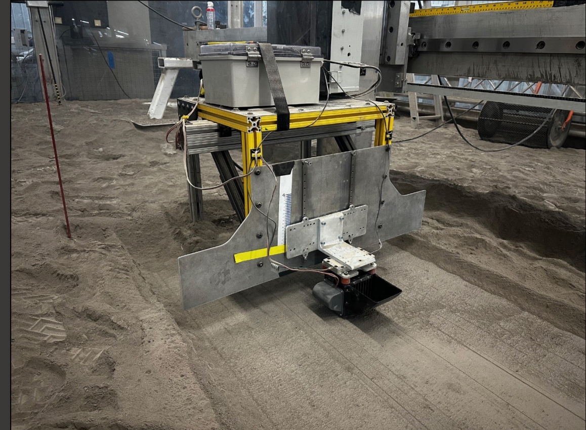
Compaction test configuration on the 2-axis gantry.
